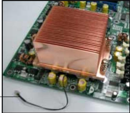
2. Hold down the heatsink lightly and twist each of the four screws with a Philips (cross) screwdriver just enough to attach the heatsink to the motherboard. When the four screws are attached, tighten them one by one to completely secure the heatsink.
