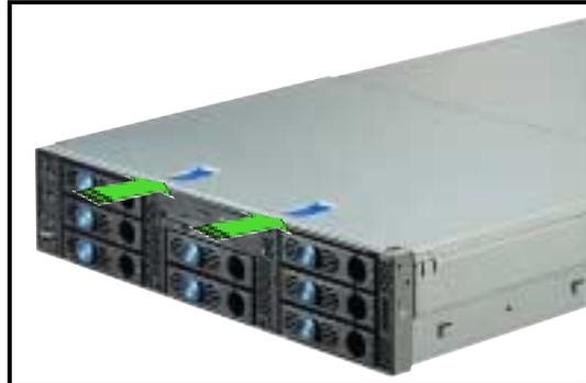
2. With both hands, flip up the front corners of the top cover then lift the front half.
