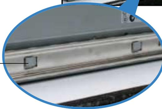
3. Secure the server rail to the chassis with a screw.
