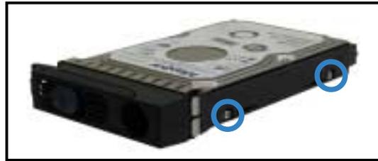
6. Carefully insert drive tray and push it all the way to the depth of the bay until just a small fraction of the tray edge protrudes.
