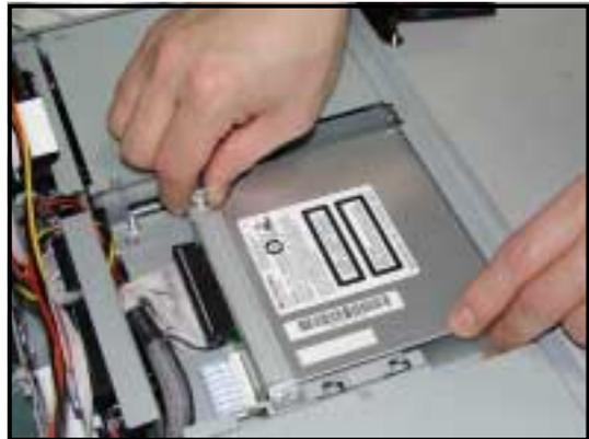
3. Slide the drive bracket toward the SCSI backplanes to release it from the chassis, then carefully pull it out of the drive bay.
