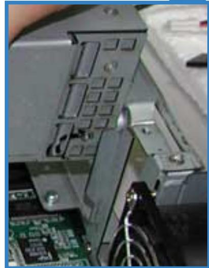
13. Match and push the cage card connector into the PCI-X slot (PCI-X2) until the PCI cage fits in place.
