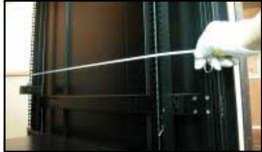
5. Take three pieces of rack rail, consisting of the middle piece, one front end (with stopper tab), and one rear end (without stopper tab). Assemble the rack rail to a length depending on the rack depth.
