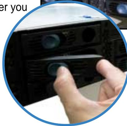
3. Firmly hold the tray lever and pull the drive tray out of the bay.
