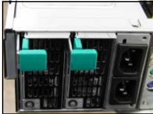
2. Hold the module lever and press the latch on the inner side to release the module.
