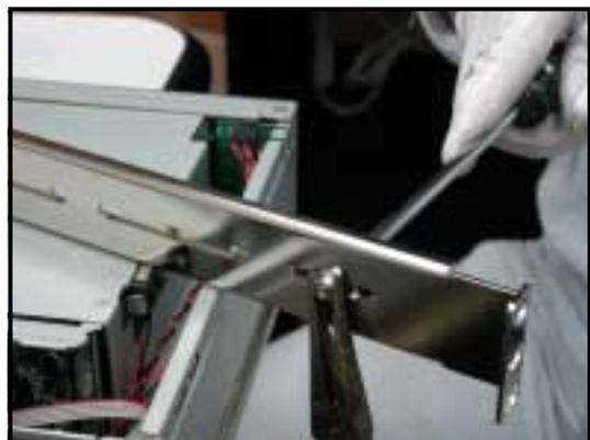
7. Measure the rack rail when assembled to make sure that it fits the rack.
