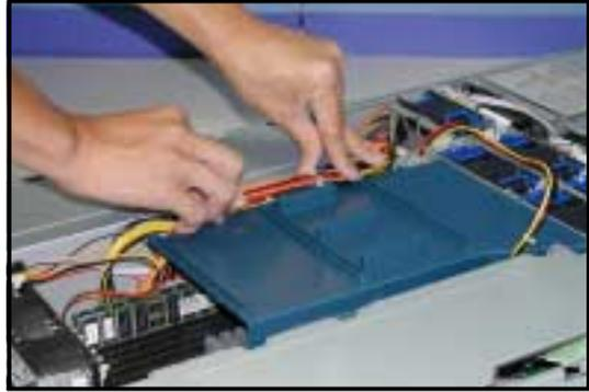
6. Flatten the power cable that runs across the air duct. When properly installed, the air duct should appear as shown.
