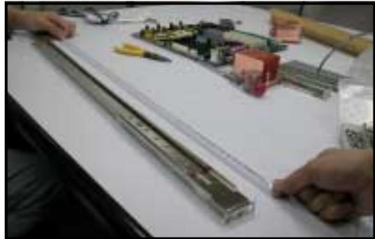
8. Position the rack rail to the 2U space on the rack.
