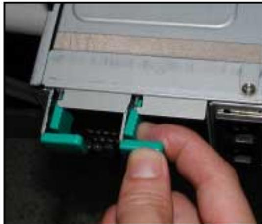
3. Firmly pull the lever to slide the power supply module out of the chassis.
