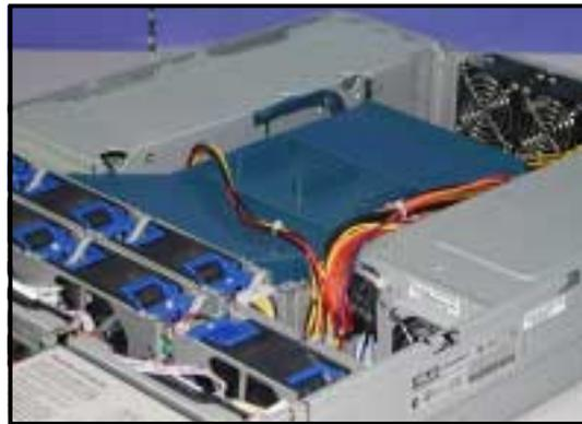
2. Hold the rear part of the air duct and press it for about a fraction of an inch, just enough to tilt the front end.
