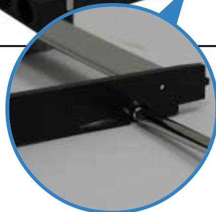
5. Place a hard disk drive into the drive tray, and secure it with four screws (two on each side).
