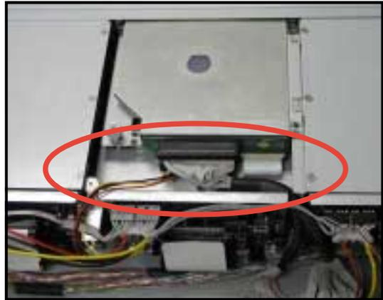
2. Loosen the thumbscrew that secures the drive bracket to the chassis. The optical drive is attached to the top of the bracket, and the floppy drive to bottom.
