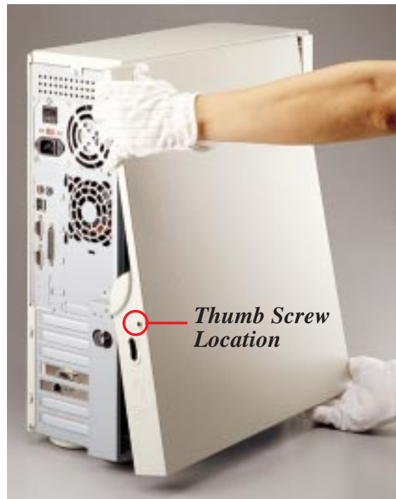
Pulling the Bottom of the Left Panel (Step 4)
