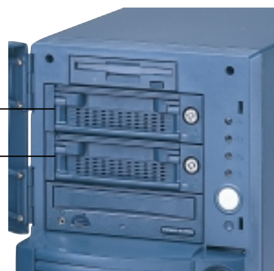
Installed Hot-Swap Drive Trays
