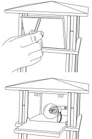
1. Use a small flat tool (like a flat-head screwdriver) to open the top of the lantern's front door.
