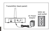
3. Connect the small, round plug from the transmitter AC power adapter to the transmitter's DC IN jack. Plug the other end of the transmitter AC power adapter into any standard 120V AC wall outlet.
