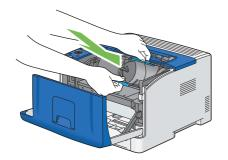
3 Make sure that the two tabs of the toner cartridge align with the grooves on the printer, and then insert it into the printer until it clicks.
