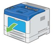
4 Grasp both sides of the bypass tray, and then pull the bypass tray from the printer.
