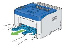
3 Slide the width guides to the edge of the tray. The width guides should be fully extended.
