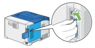
4 Slide the control board cover towards the rear of the printer and remove the cover.
