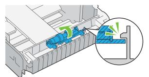
4 Load paper in the standard 250 sheet tray, and then insert the standard 250 sheet tray into the printer and push until it stops.
