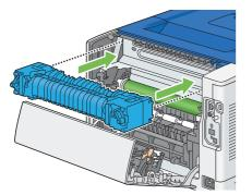
4 Lower the two gray levers to lock the fusing unit.
