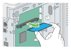
6 Align the guide on the control board cover with the slot around the control board, and slide it towards the front of the printer.
