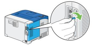
8 Reconnect all cables into the rear of the printer and turn on the printer.
