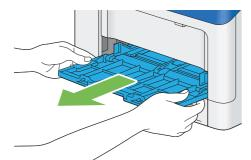
7 Pull the standard 250 sheet tray out of the printer about 200 mm.
