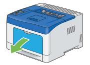
**6** Grasp both sides of the bypass tray, and then pull the bypass tray from the printer.
