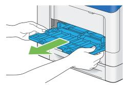
5 Pull the standard 250 sheet tray out of the printer about 200 mm. Hold the standard 250 sheet tray with both hands, and remove it from the printer.
