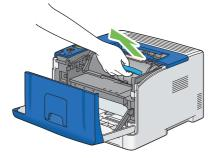
4 Grasp the handle on the front of the drum cartridge, and then pull it out halfway with one hand.
