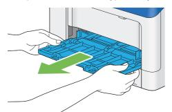
3 Pull the standard 250 sheet tray from the printer about 200 mm.
