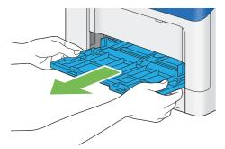
3 Pull the standard 250 sheet tray from the printer about 200 mm.
