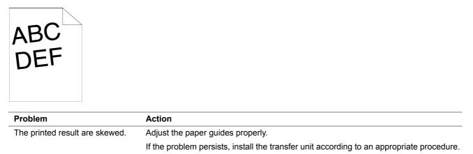
Install the transfer unit according to an appropriate procedure.
