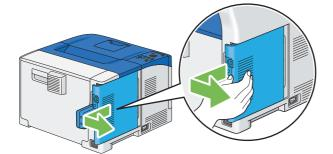
5 Remove the wireless printer adapter from the printer by releasing the adapter's hook while pushing the wireless printer adapter towards the front of the printer.
