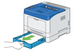
2 Hold the optional 250 sheet feeder with both hands, and remove it from the printer.
