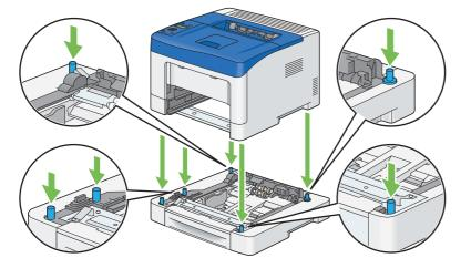
**10** Secure the optional 250 sheet feeder to the printer by tightening the two screws provided with the feeder with a coin or similar object.
