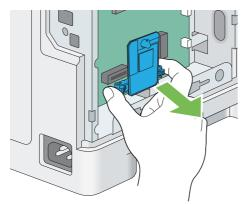
6 Align the guide on the control board cover with the slot around the control board, and slide it towards the front of the printer.
