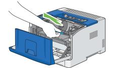
**5** Grasp the handle on the top of the drum cartridge with the other hand, and then pull it out completely.
