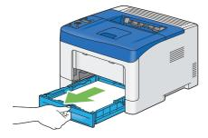
4 Hold the standard 250 sheet tray with both hands, and remove it from the printer.
