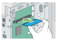
**5** Push the memory module firmly into the slot.
