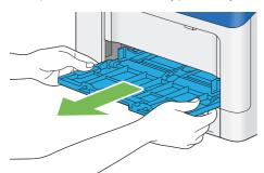
4 Pull the tray out of the printer about 200 mm.
