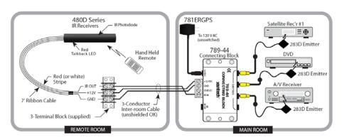
Input connections must be made as illustrated. To extend the emitter wires to a more distant location, you may splice in 2-conductor wire, in the wire gauges mentioned before, as needed.
