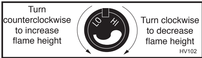
Fig. 13 Flame adjustment knob for Honeywell valve.
