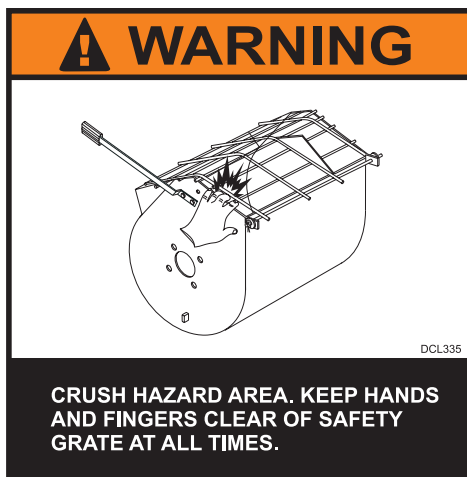
Figure 38. Safety Grate (Crush Hazard)
