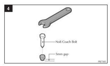
Screw in No.8 coach bolt leaving 5mm gap from the surface of the floor.
