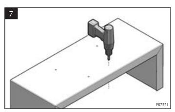
Drill four Ø8mm holes. Straight through both 7. sides.
