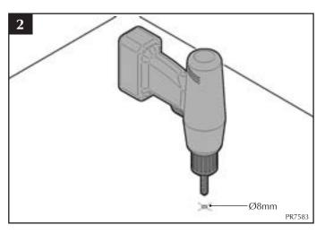
Remove bench and drill the two marked positions with Ø8mm hole to 50mm deep.
