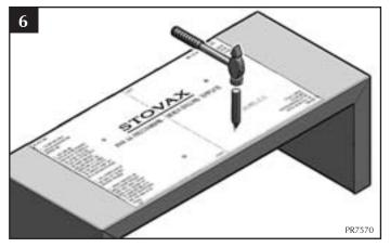
Mark drilling points with a centre punch. 6.
