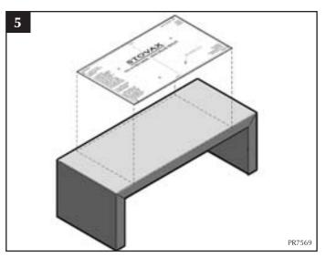
Slide The bench over the coach bolts and tighten. Position drilling template as you would the stove.
