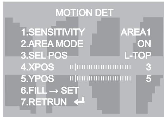
1) When the SPECIAL menu screen is displayed, press the Function Setup switch so that the arrow indicates 'MOTION DET' .
