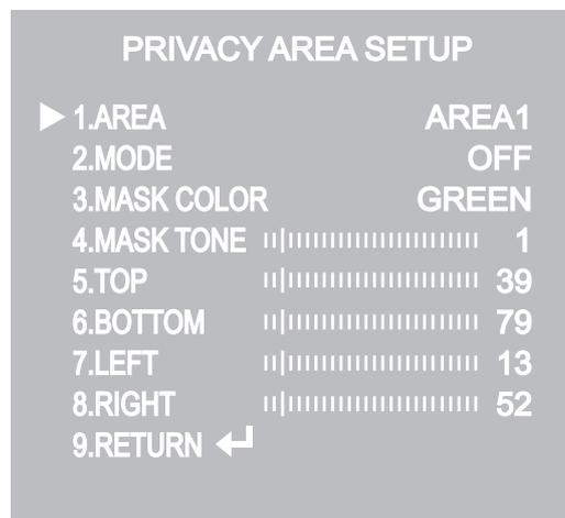
1) When the SPECIAL menu screen is displayed, press the Function Setup switch so that the arrow indicates 'PRIVACY'.
