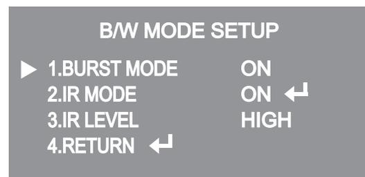
◆ **AUTO** : The mode is switched to 'Color' in a normal environment, but switches to 'B/W' mode when ambient illumination is low. To set up the switching time for AUTO mode, press the Function Setup switch. You can turn on or off the burst signal on B/W mode.
