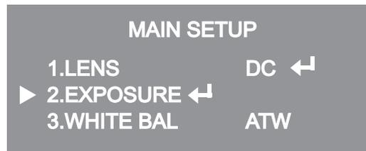
1. When the SETUP menu screen is displayed, select 'EXPOSURE' by using the Function Setup Switch.
