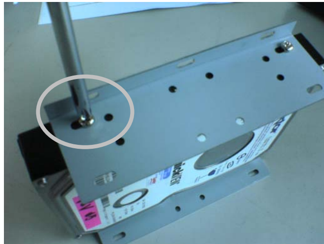
Figure 5: Attach the HDD to the bracket
