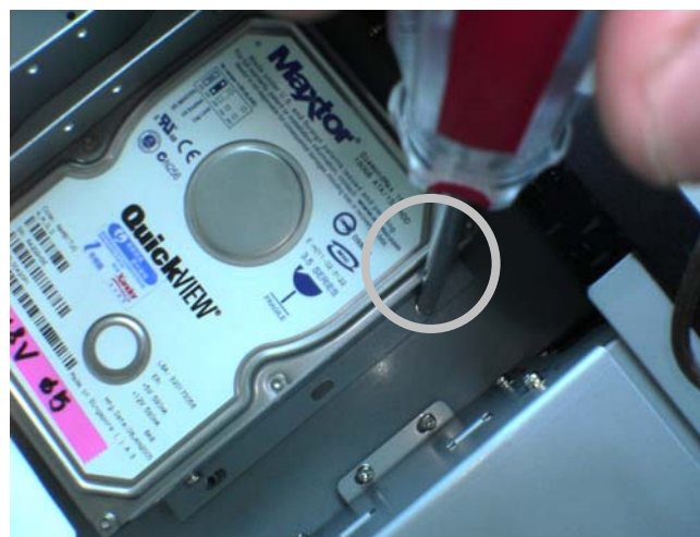
Figure 9: Attach the bracket to the DVR
