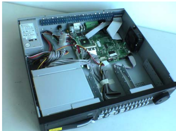
Figure 2: Internal construction of DVR-4TN/8TN/16TN/16TS/16TT
