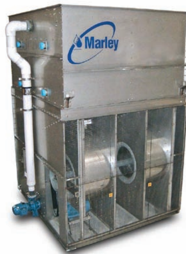
Marley MC Fluid Cooler —Forced draft, counterflow design. G-600 galvanized steel factory assembled structure. Also available in 300 series stainless steel. The ideal solution for sound- and space-sensitive applications. CTI Certified.
