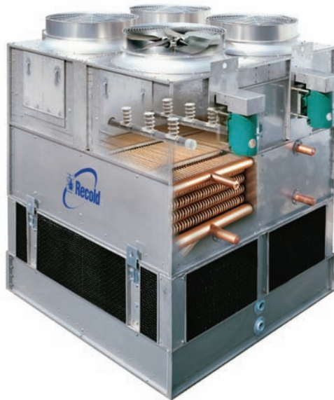
Recold MC Evaporative Condenser —Induced draft, counterflow design. G-600 galvanized steel factory assembled structure. Also available in 300 series stainless steel. Proven copper coil technology.
