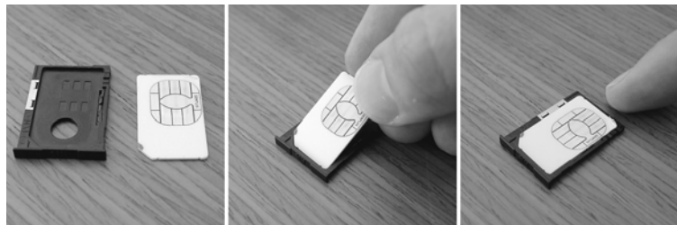
Figure 3-10: Placing a SIM card into the sled.
