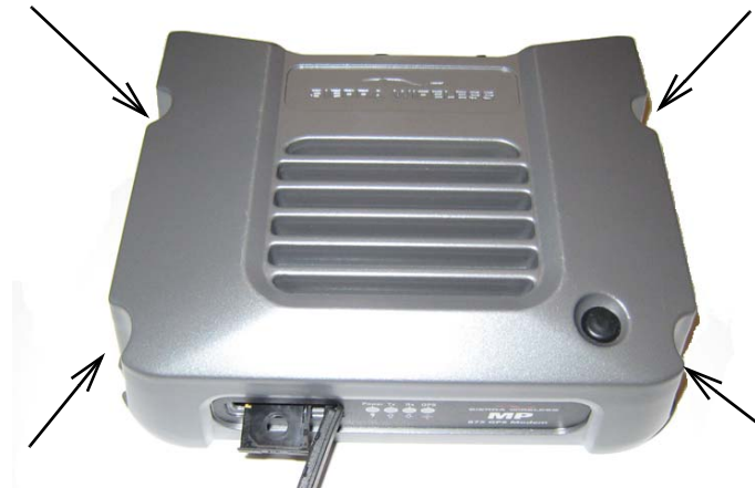
Figure 3-3: Mounting the MP modem. Arrows indicate the mounting holes. The front cover is open for illustration purposes only. Close it before mounting.
