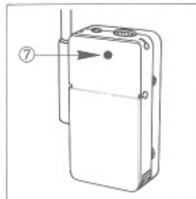
Potentiometer for adjustment of attenuation
