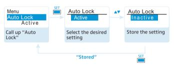
The lock mode prevents that the plug-on transmitter is accidentally switched off or programed during operation. The lock mode icon S G on the current standard display indicates that the lock mode is activated.
