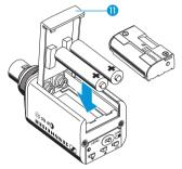
Close the battery compartment. The battery compartment cover 1 locks into place with an audible click.
