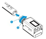
Tighten the locking ring 2 in the direction of the arrow.
