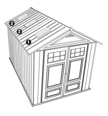
The Skylight Roof Panel can be assembled in 1 of 3 different positions. Assembly instructions show the Skylight Roof Panel being assembled in postion 2.
