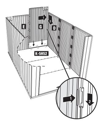
Engage lap joint between Left Back Panel (E) and Right Back Panel (G) and install Wall Connectors (Q) 4 places.
