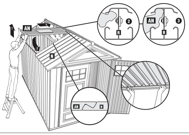
Lubricate roof snaps on left side of the back Gable (M) 4 places.
