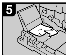
6. Remove misfed paper. 7. Close the Z3 cover. 8. Put the duplex unit back. 9. Close the front cover.
