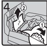
4. If you cannot remove the misfed original, turn the dial ① clockwise and remove the misfed original ②.
