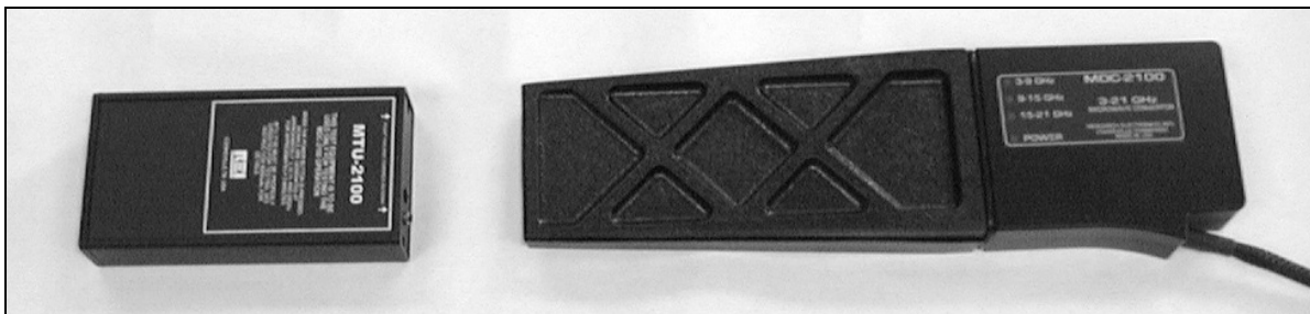
Figure 12: PROPER MTU ORIENTATION FOR TESTING BAND 1 (3- 9GHZ) OR MDC- 900
