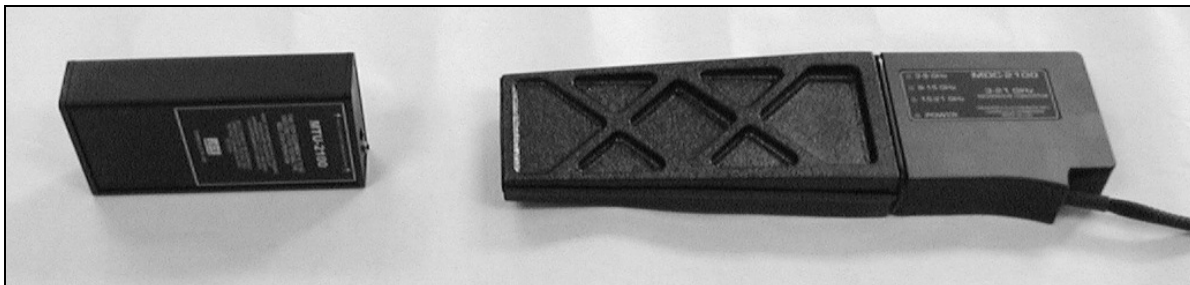
Figure 13: PROPER MTU ORIENTATION FOR TESTING BAND 2&3 (9- 21GHZ) FOR MDC- 2100 ONLY
