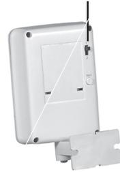
Mount your Motion Detector on a wall at a height of five to six feet, using the mounting bracket and screws provided.
