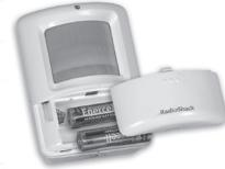
Press and hold the **TEST** button on the back of your Motion Detector for three to four seconds, and then release it. This initializes your Motion Detector and picks a random code that is used when it is registered with your Security Console. Place the unit face down, so it won't detect any motion during the registering process.
