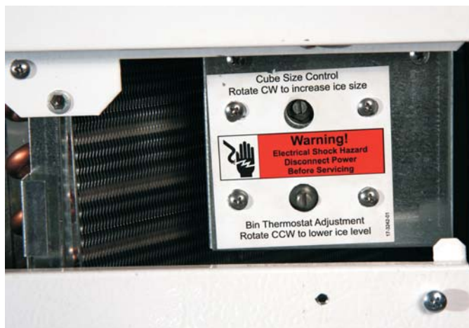
Condenser and Bin Thermostat
