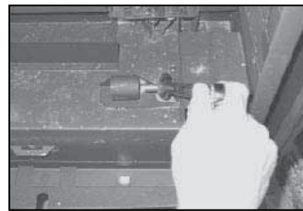
Figure 6.4 Remove the main burner orifice using a 5/8 in. wrench. Replace orifice with the proper size as indicated for your gas type and venting.
