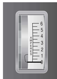
Figure 8. Ammeter Indicates Battery Is Fully Charged
