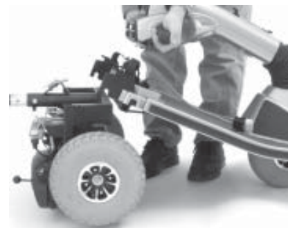
Figure 20. Separating The Frame Sections
