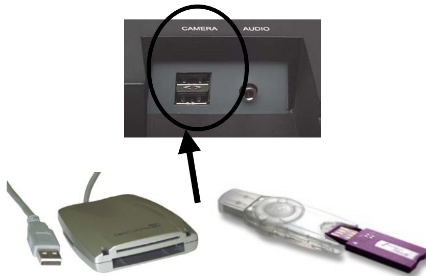
Figure 15 – Connecting a Card-Reader or Thumb-drive
