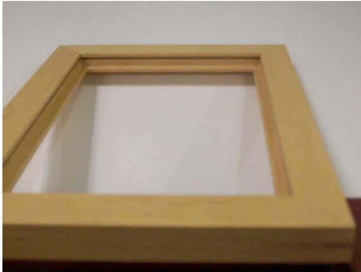
Figure 23 – Example of groove in rear of frame
