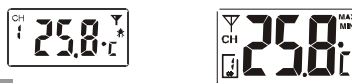
Transmitter's low battery indicator (shows on the transmitter) Transmitter's low battery indicator (shows on the main unit)
