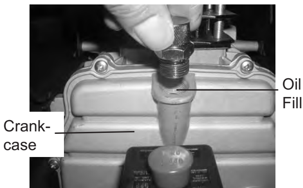
Figure 3. Installing the Oil & Oil Breather Cap
