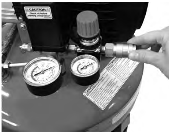
Figure 3. Installing the Air Chuck
