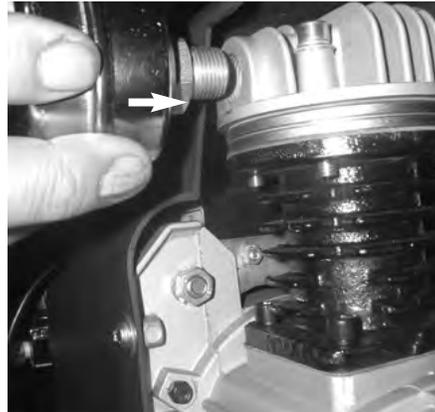
**Figure 4.** Installing the Air Filter
