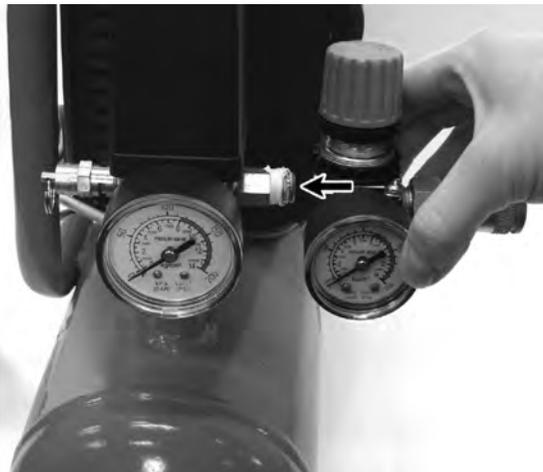
**Figure 3.** Installing the Air Regulator
