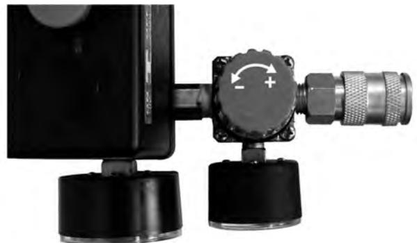
Figure 6. Adjusting the Air Pressure
