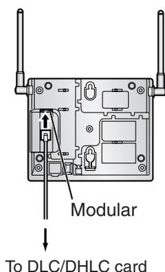
5. Install the CS temporarily for the site survey. Install the CS at least 2 m above the floor, keeping the antennas in the upright position.
