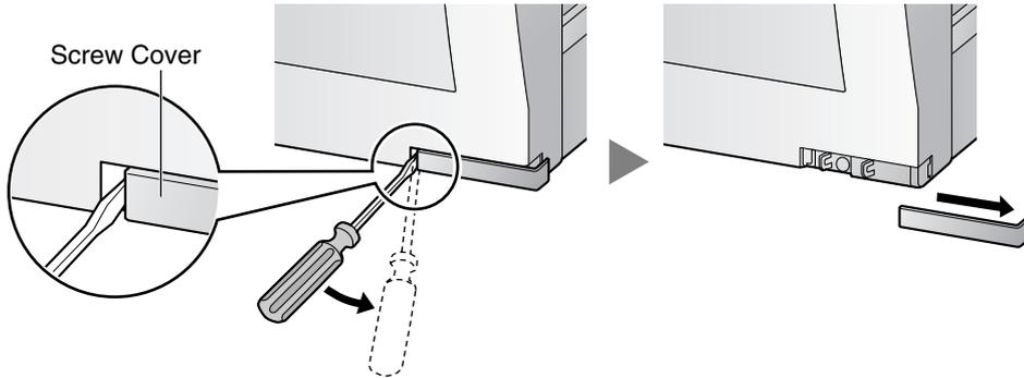
2. Turn the screw anticlockwise to loosen.
