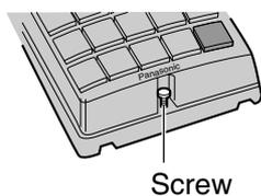
2. Pass the wires through the hole in the base cover, and attach the base cover to a wall using 2 screws.
