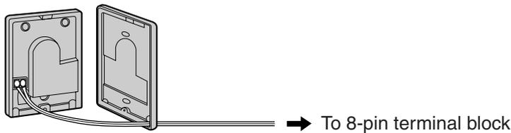
4. Re-attach the 2 halves and re-insert the screw.
