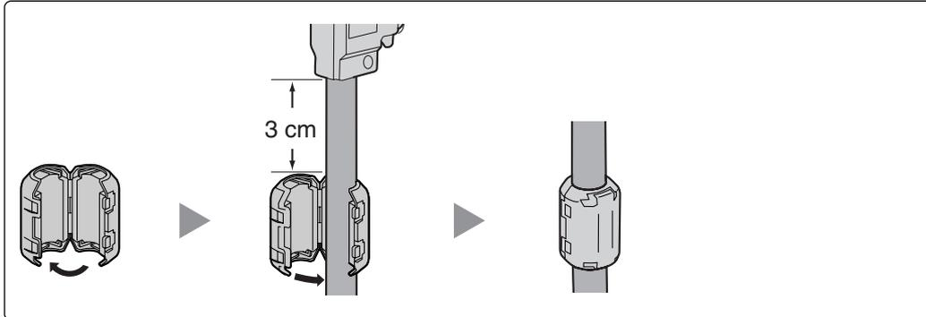
If you need to open the ferrite core, use a flathead screwdriver to unlatch the case of the ferrite core.
