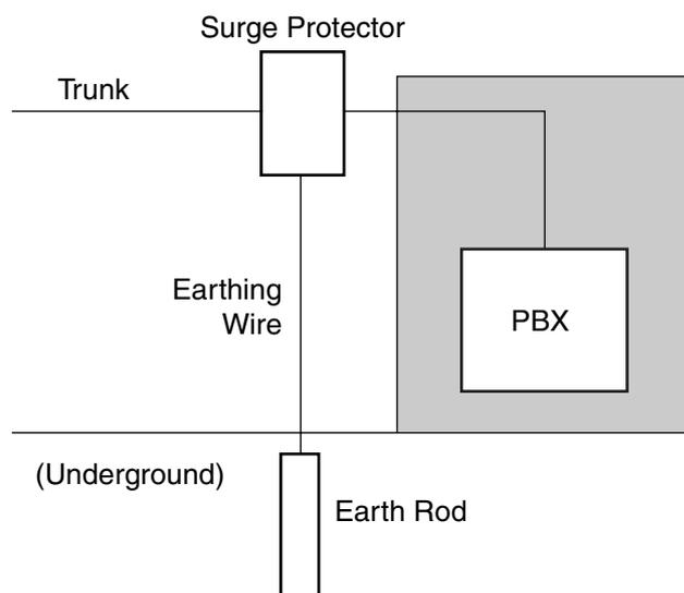
1. Connect the earth rod to the surge protector using an earthing wire with a cross-sectional area of at least 1.3 mm<sup>2</sup>.
