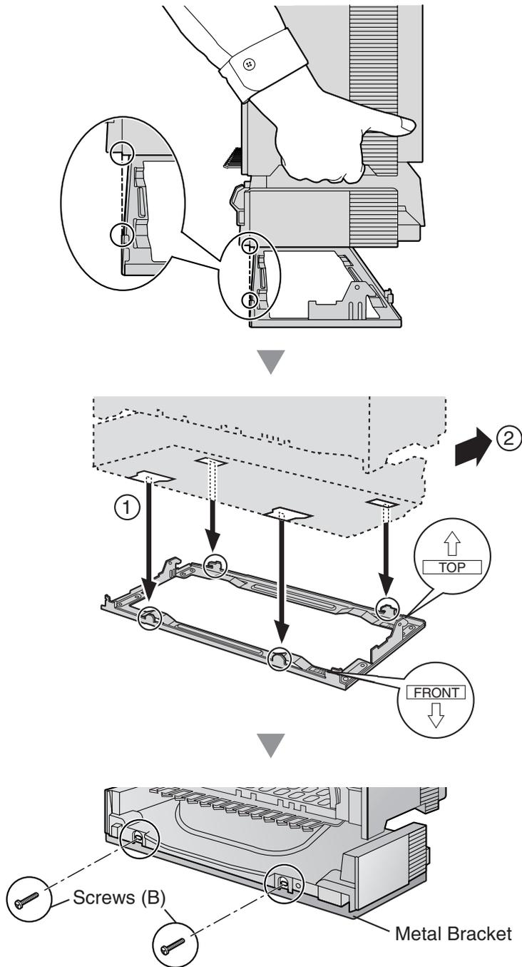
4. Fix the front cover on the shelf (refer to "3.2.3 Opening/Closing the Front Cover").
