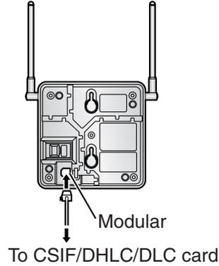
2. Pass the cable through the groove of the CS (in any direction depending on your preference).
