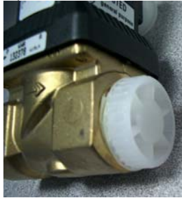
Photo 8. \frac{3}{4} ” Plug in Automated Drain Valve
