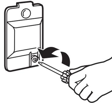
3. Turn bulb counterclockwise. Replace the bulb with a 10-watt appliance bulb only. Replace the cover and secure with the screw.
