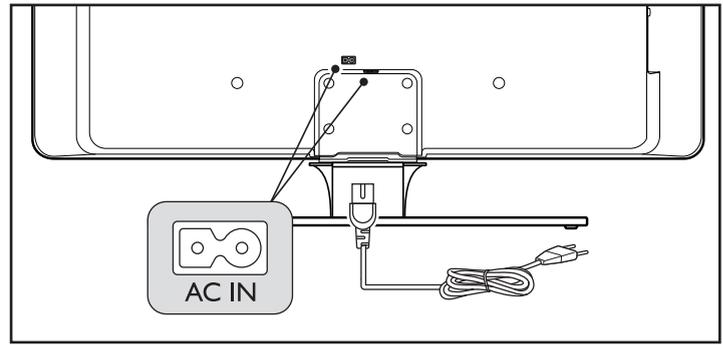
2. Insert the power cord fully into the TV power connector.
