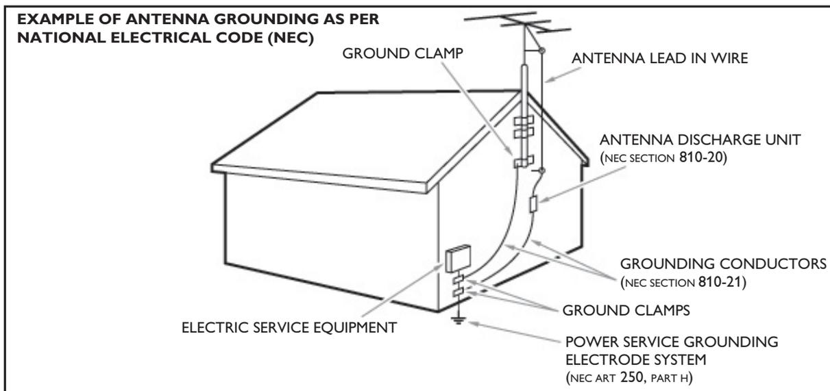
**Note to the CATV system installer:** this reminder is provided to call the CATV system installer's attention to Article 820-40 of the NEC that provides guidelines for proper grounding and, in particular, specifies that the cable ground shall be connected to the grounding system of the building, as close to the point of cable entry as practical.
