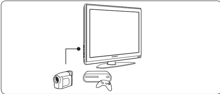
Use the TV side connectors to connect to mobile devices such as a high definition game console. You can also connect a pair of headphones.
