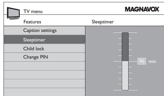
2. Press **▲** or **▼** to select a value from **0** to **180** minutes. For example, when you select **90**, the TV switches to standby in 90 minutes.
