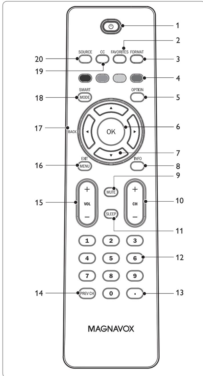
1. Switches the TV on from standby or back to standby. The TV is never powered off completely unless it is physically unplugged.
