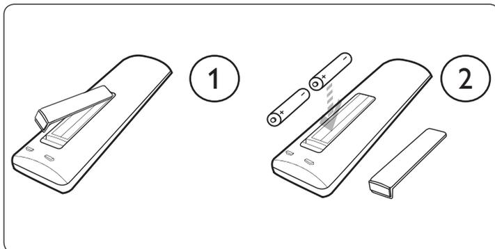
1. Open the battery cover on the back of the remote control.
