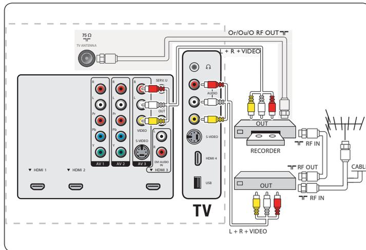
If your recorder has an S-VHS video jack: for improved picture quality, connect an S-Video cable with the S-Video input and connect the audio cables to the audio L and R input jacks of AV3/side AV.
