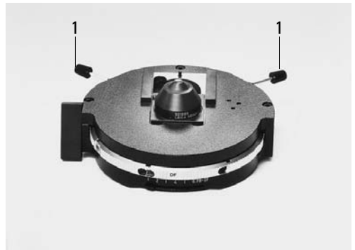
Fig. 29 Phase contrast centering procedure
