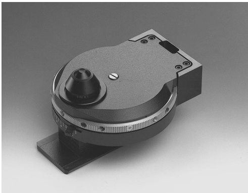
Fig. 11 Condenser 0.90 S1 (bottom up)
