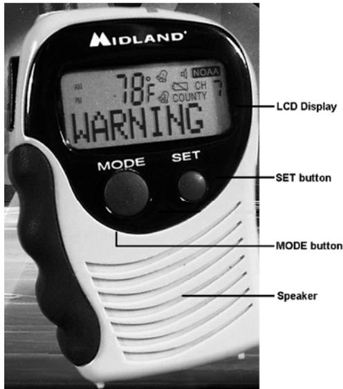
**Mode** – This is a push button that switches the display from time, date and temperature display to alarm display. Also is used to change the active county.
