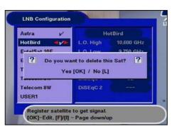
To remove a satellite, select the "LNB configuration" menu, move the cursor bar
