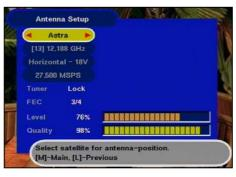
This menu is intended solely for service purposes and, if need be, i.e. if no measuring instrument is available, it can be used to align the antenna (satellite dish).
