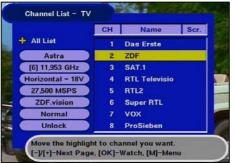
transmission frequency, polarisation, symbol rate and scrambling. The programme number, the programme broadcaster and the type of reception signal (analogue/digital) is shown on the right.
