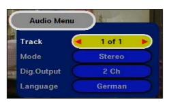
Press the button to call up the audio menu for sound and language selection. You can now make the required settings, e.g. language selection, provided the corresponding data is contained in the reception signal (sound track), Dolby Digital (5.1 CH). Select the menu points by
