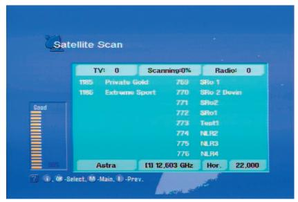
During scanning, the signal quality, the scanning progress and the new channels found are displayed. At the end, you will see a message to tell
