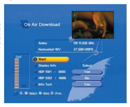
The current reception situation is displayed here (satellite, transponder, frequency, symbol rate, polarisation). Use the
