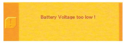
You can continue to operate the sytem, but there may be communication errors between the UFD 170 and the turntable (e.g. for satellite search).
