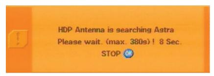
If a signal is found, the antenna automatically goes into the fine tuning mode (max. 90 seconds, if signal is adequate, the position is immediately saved).
