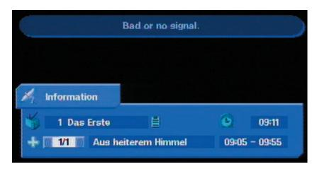
"Weak or no signal" indicates that an error has occurred in the receiving system or in the receiver settings, or that the transponder is not sending. The channel message then shows a satellite antenna instead
