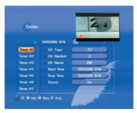
Use the keys to move the cursor to the desired timer and confirm with .
