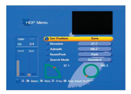
Use the keys to go to the "Reset/Park" option, and change the selection to "Reset" using the keys. Now press The following screen appears:
