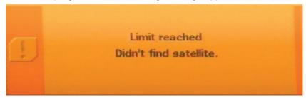
press and start satellite search with a different programme of the same satellite and check whether there are any obstructions to the antenna's reception.
