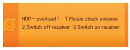
If this message appears, check the turntable and antenna to ascertain whether the system is blocked by an object (e.g. a branch) or whether the on-board voltage is too low. Proceed in the sequence shown above (screen).
