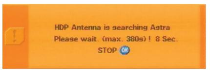
As soon as the turntable has found the correct satellite, automatic fine-tuning is carried out. The search lasts a maximum of 90 seconds (if the signal level is sufficient, the satellite position is immediately saved by the turntable unit). The screen may "freeze" during fine tuning - this is determined by the system.
