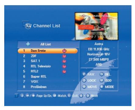
At the top left is a "+" for the complete list. In the column below it, you will see details of the channel name, the channel number and whether the programme is a favourite, locked or encrypted.
