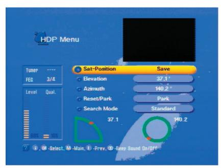
You can correct the inclination and horizontal angle of the antenna using the "Elevation" and "Azimuth direction" settings. To do this, press
