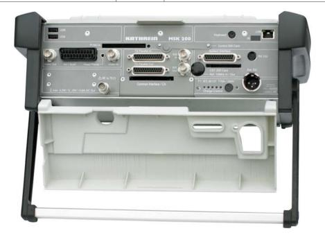
The illustration shows the MSK 200/S2 21710024 with 75- $\Omega$ -BNC socket; another version is available, MSK 200/S2 21710025 with 50- $\Omega$ -N socket.
