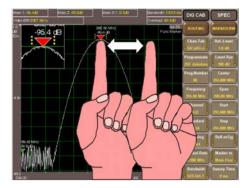
To open the zoom window, press and hold your finger on the marker; you can then shift it to the desired position!
