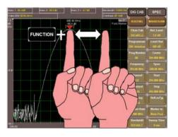
Press the "FUNCTION" key, tap on the screen and hold to drag the screen section as required (e.g.: the delay time on the oscilloscope, the mid-frequency on the spectrum analyser)!
