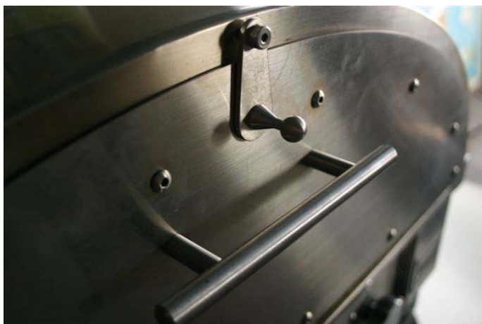
Safety Latch – Be sure to wear heat-resistant mitts or gloves, and use two hands when opening and closing the door.
