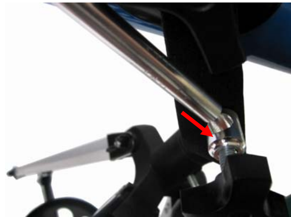
Figure 8. Put the rod through the eyebolt on mount
