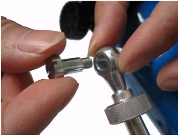
Figure 6. Install Altitude adjustment rod
