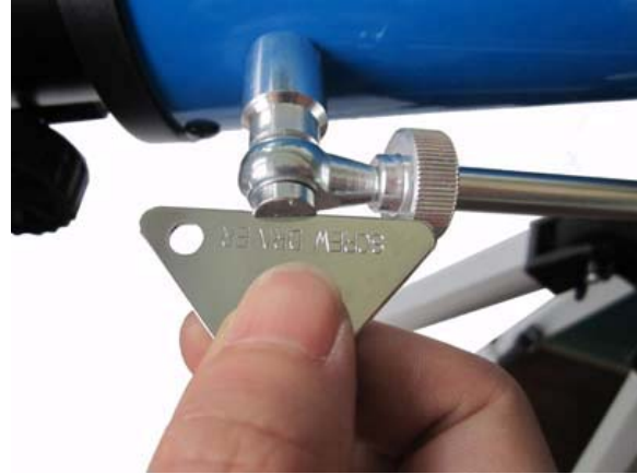
Figure 6. Install Altitude adjustment rod
