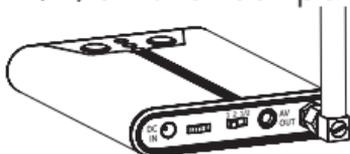
The receiver must be set to the '1/2' position to allow two cameras to be monitored. The next step will be to set the channel selection switch on both cameras. **See Camera Channel Selection.**
