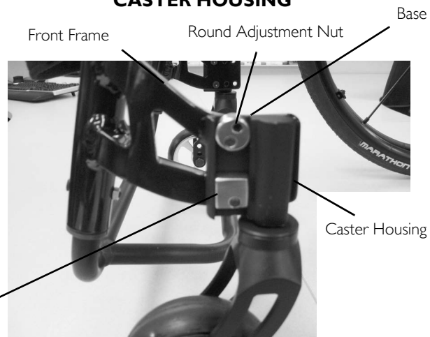
FIGURE 5 Repositioning the Front Caster Housings
