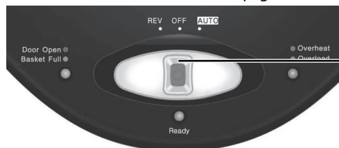
Emergency stop switch (ESS)
