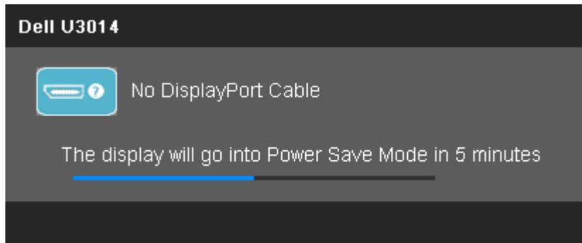
4. This box also appears during normal system operation if the video cable becomes disconnected or damaged.
