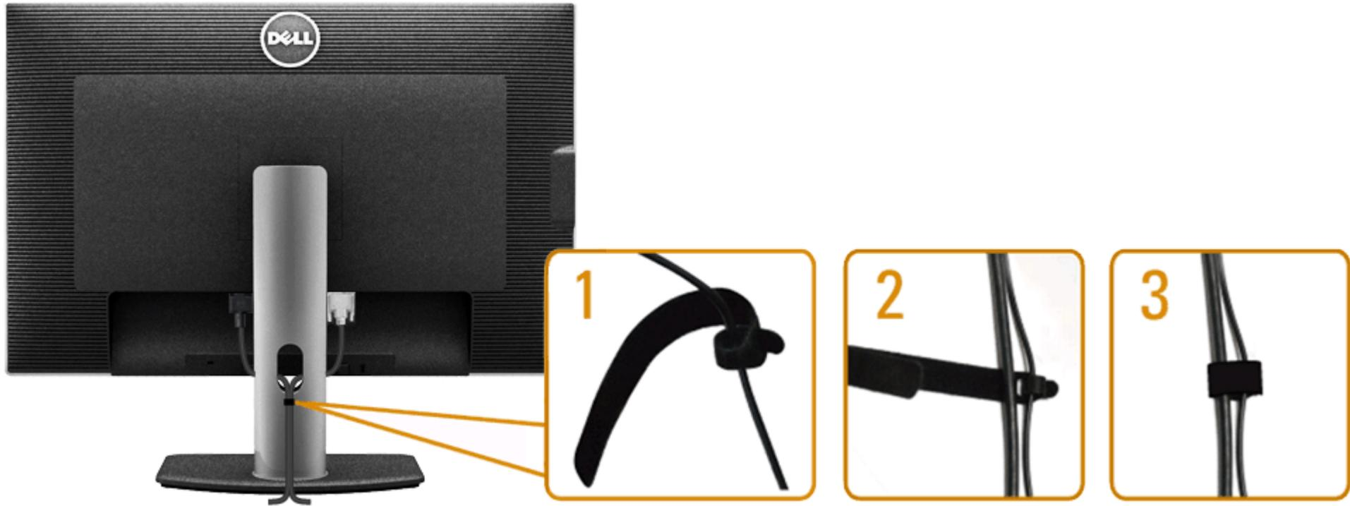
After attaching all necessary cables to your monitor and computer, (See [Connecting Your Monitor](#) for cable attachment,) use the Velcro cable tie to organize all cables as shown above.
