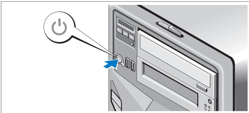
Press the power button on the system and the optional monitor, if used. The power indicators should light.
