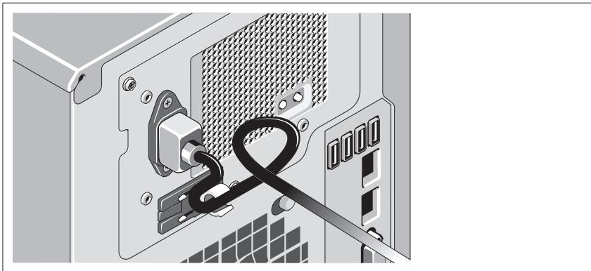
Bend the system power cable into a loop as shown in the illustration and secure the cable with the provided strap.
