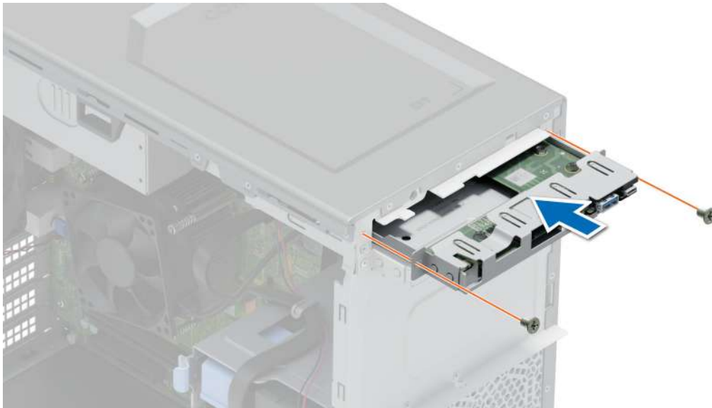
Figure 62. Installing the control panel cage
