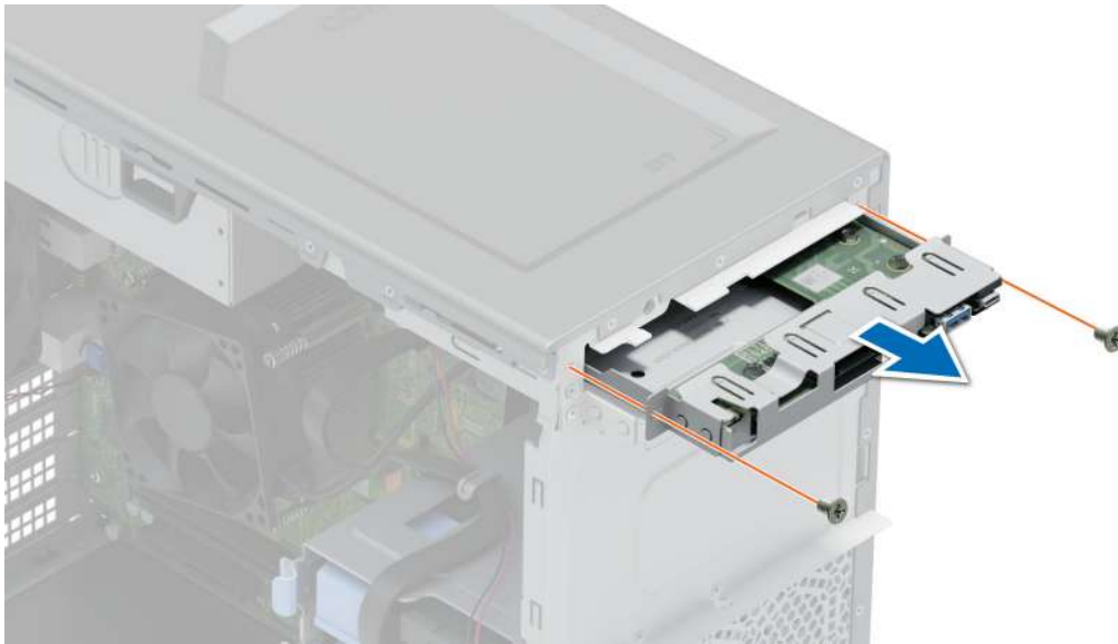
Figure 59. Removing the control panel cage
