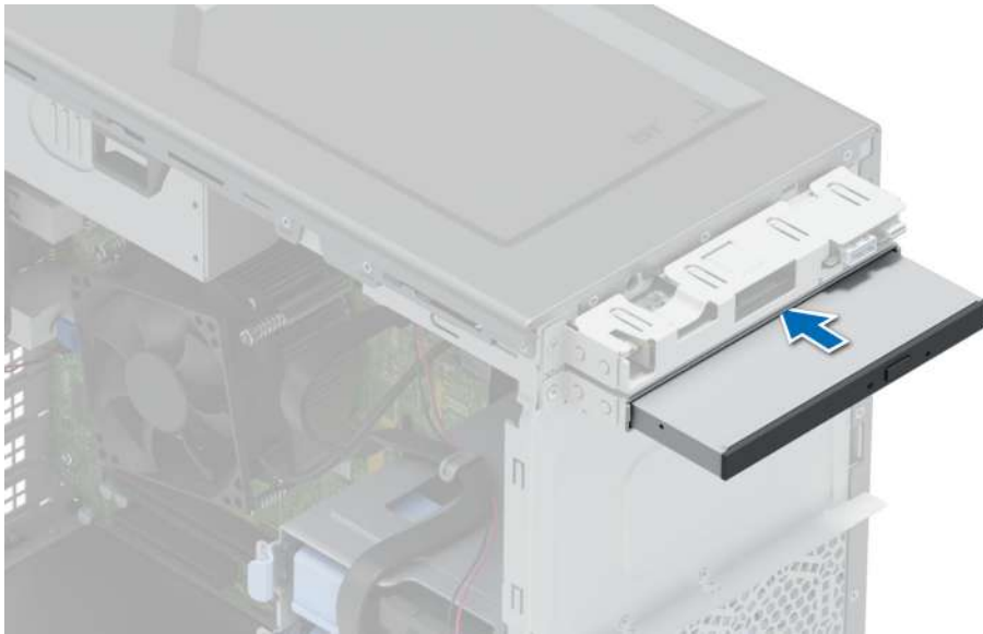
Figure 27. Installing the optical drive
