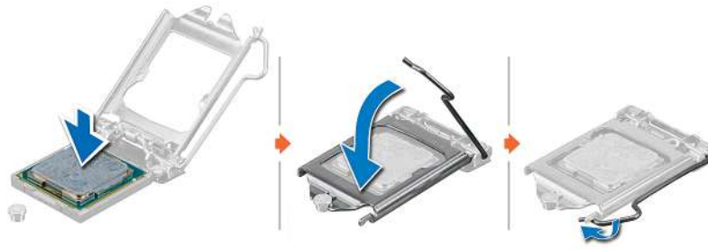
Figure 45. Installing the processor
