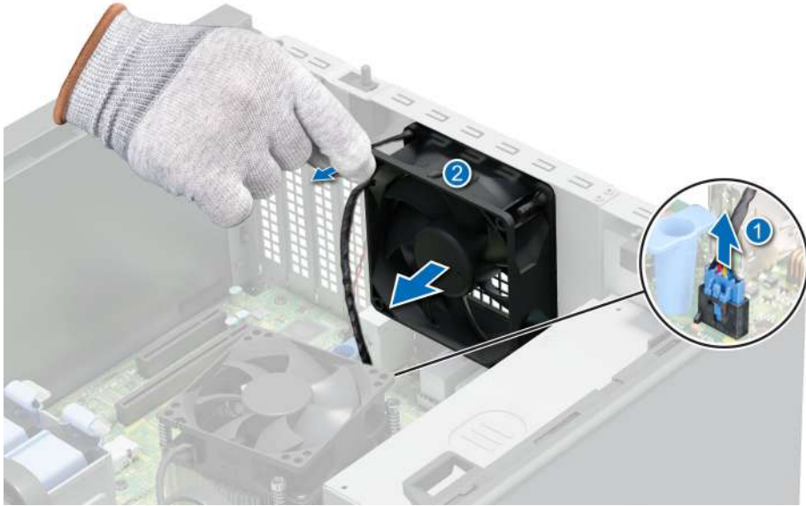
Figure 32. Removing the cooling fan
