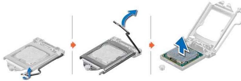
Figure 44. Removing the processor
