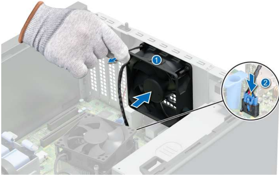
Figure 33. Installing a cooling fan
