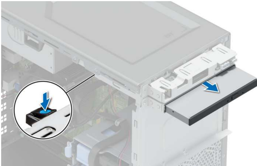
Figure 26. Removing the optical drive
