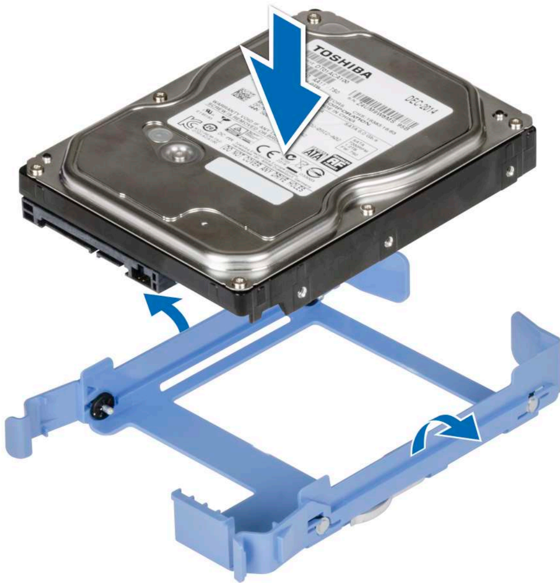
Figure 15. Installing a drive into the drive carrier
