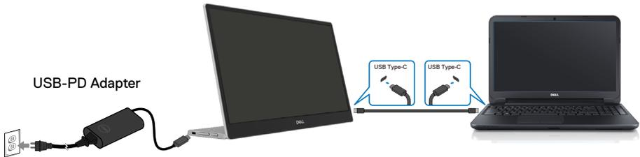
2. Connect Type-C power adapter to C1422H and connect C1422H to the mobile phone with a USB Type-C cable.
