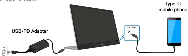
**NOTE:** When you encounter abnormal charging condition, please check your power capacity of power adapter connected with C1422H and make sure it is enough for C1422H and other devices. In order to use the monitor smoothly, please refer to the [Preset display modes](#) and [Power management](#).
