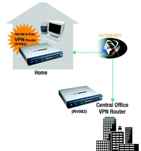
Figure 2-1: VPN Router-to-VPN Router VPN
