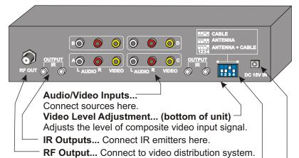
Used to set the channel mode of the modulator. **Power Input...** Connect Power supply here.
