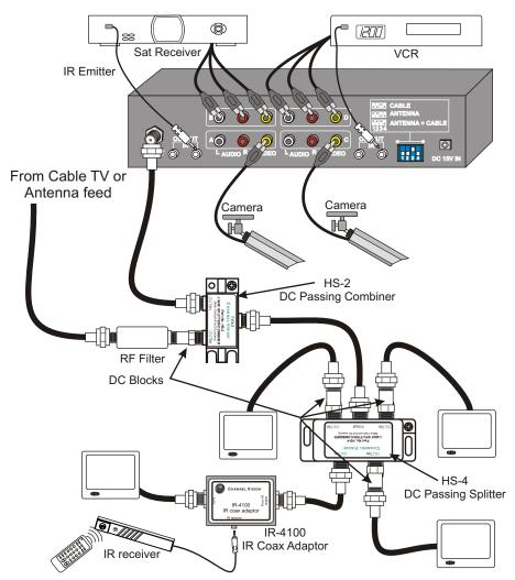
The modulator supports Channel Vision's IR over coax technology allowing up to 8 IR-4100 IR coax adaptors to be installed in the system. Standard IR receivers can be connected so that IR signals are transmitted back to the modulator where the IR emitters will flash the signals into the source devices. This enables you to control your source devices even though they are in a different room.
