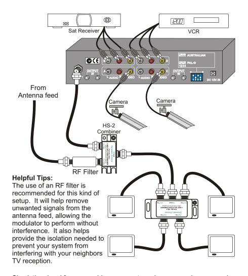
Check the signal from your video sources to make sure you have a good picture before connecting to the modulator. Connect the RF output from the modulator as shown in the diagram above.
