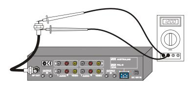
If you are trouble shooting a whole-house IR system and you measure approximately 8-12 Volts DC on the output of the Modulator, but 0 Volts DC on the output of your RF splitter, check the following items:
